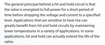
Clippard's hit and hold option minimizes the heat generated by the coil when the valve is energized for longer than 5 minutes. The optimized duty cycle is factory set and is available on Clippard NIV, PIV, and NPV series valves.
